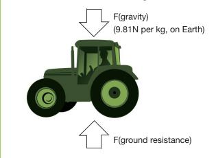
The force of gravity on Earth is 9.81 N for every kilogram of the object's mass. The force of gravity on other planets varies according to the size of the planet, which determines its gravitational force.
