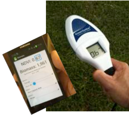
Figure 3 The relatively new Trimble Greenseeker Handheld can be calibrated to measure the green fraction of a pasture sward.
