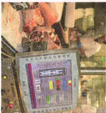
Each carcass is x-rayed and that information is used to guide the robotic cutter with millimetre-perfect accuracy.
