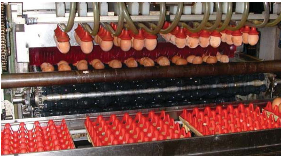
Figure 7 – Eggs loading matching in an egg processing plant. Source: International egg commission, 2013
