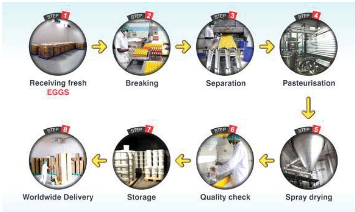
Figure 5 – Egg processing cycle. Source: Eggway, 2011
