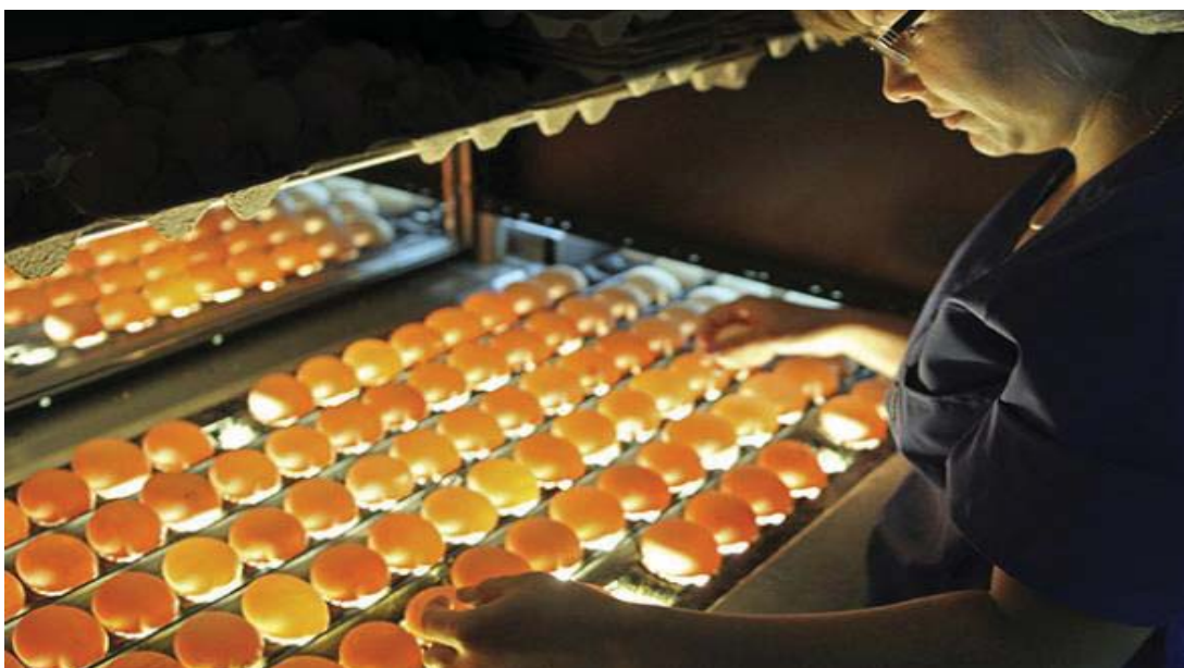
Figure 9– Egg candling process in an egg processing plant. Source: International egg commission, 2013
