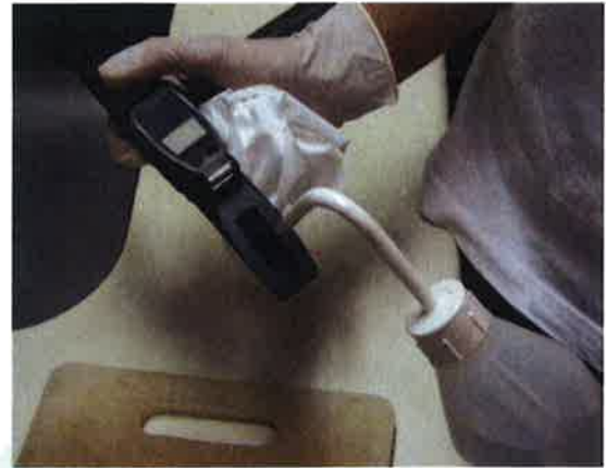
Figure 7. The refractometer is cleaned of fruit juice using water and dried with a soft tissue between each measurement.
