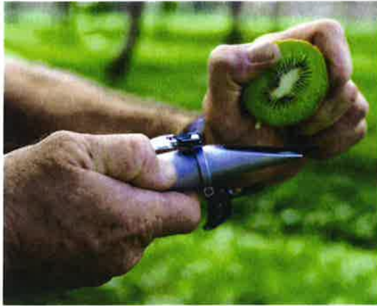
Figure 5. Juice is squeezed from either the stem or blossom end fruit slices onto the refractometer prism surface and the prism cover closed.
