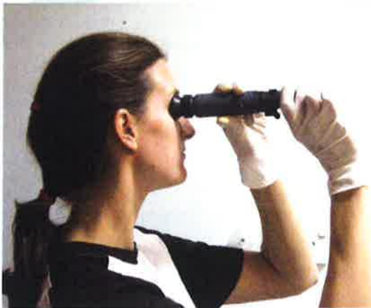
Figure 6. The Brix measurement is seen through the eye piece once the refractometer is pointed towards a light source. The eyepiece may need to be focussed to suit the operator.
