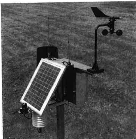
Automatic stand alone weather stations like this Harvest Standard model present live data from the Harvest web page on computer or smart phone. (Photo supplied by Harvest).
