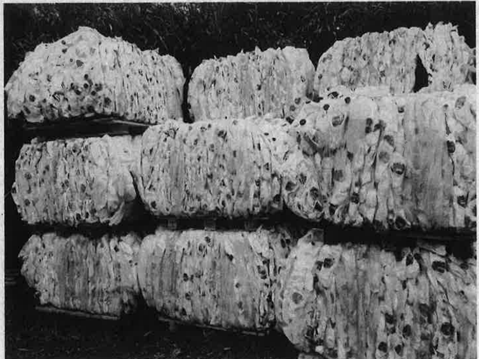
The waste plastic arrives at the factory in bales before being cut into fine chips and mixed together, fed into an extruder and then into the mould machine that makes the posts.
