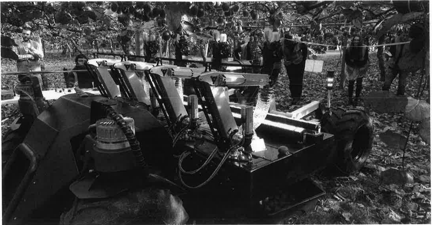
The Robotics Plus team has developed a prototype robot to help pick some of the more than 3 billion kiwifruit harvested in New Zealand each year
