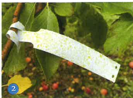
① Water sensitive papers turn blue when spray droplets come into contact and are a good tool for evaluating spray coverage, ② Yellow dye tracer was used to measure how much spray was deposited on leaves or 'artificial leaves' (plant tags), ③ Samples were rinsed in water to extract the dye then measured on a spectrophotometer
