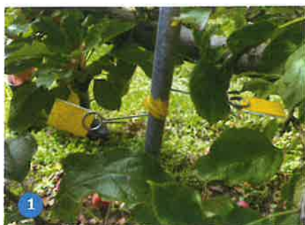
① Water sensitive papers turn blue when spray droplets come into contact and are a good tool for evaluating spray coverage, ② Yellow dye tracer was used to measure how much spray was deposited on leaves or 'artificial leaves' (plant tags), ③ Samples were rinsed in water to extract the dye then measured on a spectrophotometer
