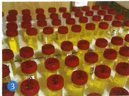
① Water sensitive papers turn blue when spray droplets come into contact and are a good tool for evaluating spray coverage, ② Yellow dye tracer was used to measure how much spray was deposited on leaves or 'artificial leaves' (plant tags), ③ Samples were rinsed in water to extract the dye then measured on a spectrophotometer
