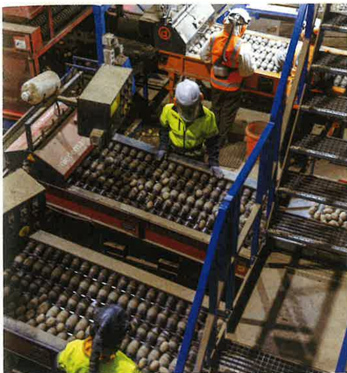
Graded seed potatoes head down the lines to the cutting machine
