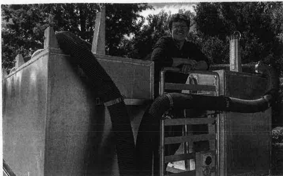
Dr Suzanne Rowe with a Portable Accumulation Chamber, which tests methane emissions of the extremely high and low-emitting bulls' progeny.
